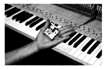
make the key move the specified amount. The tool is a dial indicator, attached to a metal base with enough weight to depress each white key. An arm extends from both sides of the gauge and rests on the top of the adjacent keys to the one being measured. These arms move the needle on the dial. The face of the dial displays the color and the number of paper punchings that need to be inserted or removed.
