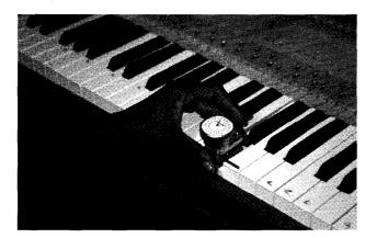
height is a subject for another article. This time we will cover the second part: creating the correct amount of downward key movement from a pre-established key height. The pictures show a unique measuring tool that makes it simple to measure the present movement of a key, and shows the technician the change that needs to be made to
